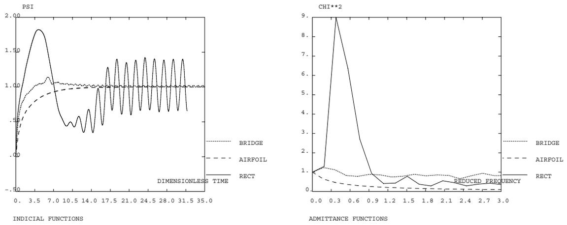
Figure 1: Aerodynamic functions
